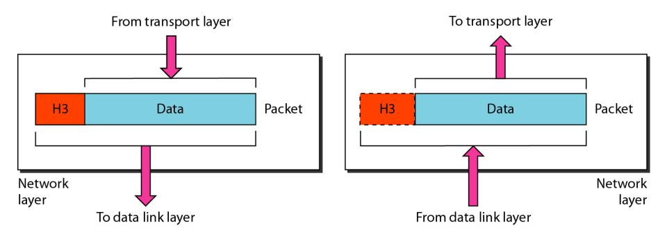
The network layer is responsible for the delivery of individual packets from the source host to the destination host.
